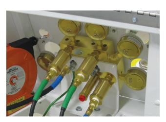
Check valves prevent backfilling and loss of pressure and media
