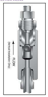
Protects pressure gauges and pressure instrumentation from surges in flow or sudden venting in the event of line failure.
