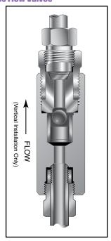
Prevents reverse flow where **leak-tight shut-off is not mandatory**. When differential drops below cracking pressure, valve closes. With all-metal components, valve can be used up to 1200°F (649°C). See Technical Information section for connection temperature limitations. (Not for use as a relief valve.)
