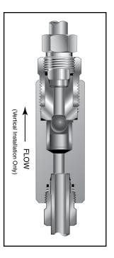
Protects pressure gauges and pressure instrumentation from sudden surges in flow or venting in the event of line failure.
