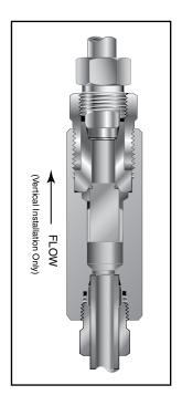
Protects pressure gauges and other pressure instrumentation from sudden surges in flow due to operator error or line failure. This valve provides dependable, tight shut-off.
