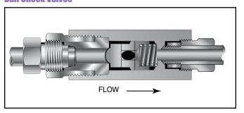
Minimum operating temperature for standard ball check valves -110°F (-79°C).
