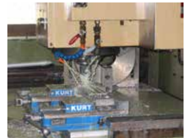
CNC Machining of ST-1600 Cover
